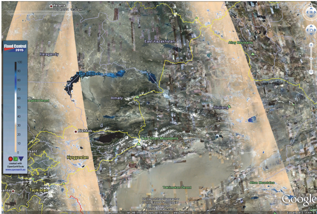
Fig. 5. Water probabilities plotted in Google Earth, collected over 24 h from 5–6 October 2011 over an example location in Kazakhstan. In the more transparent pixels the ability of the GFO algorithm to distinguish dry land from water, expressed in the quality indicator q , is lower.
